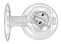
To remove the fuel cap, turn it slowly counterclockwise. The fuel cap has a spring in it; if the cap is released too soon, it will spring back to the right.
